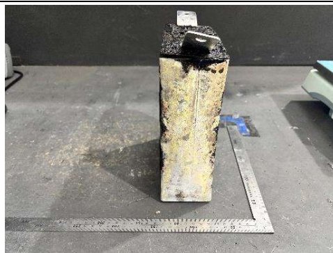
Figure 14: After thermal runaway-3
