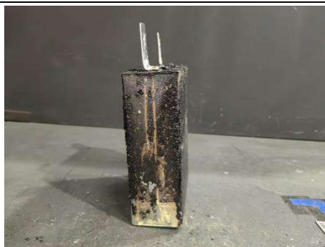
Figure 26: After thermal runaway-3
