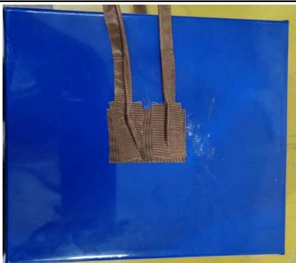
Figure 4: TC location on cell wide surface
