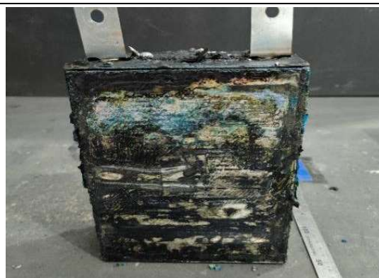
Figure 36: After thermal runaway-1
