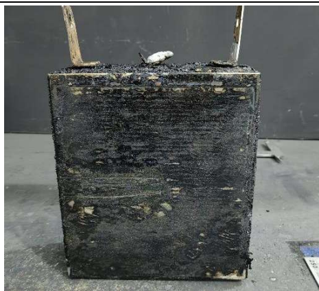
Figure 19: After thermal runaway-2
