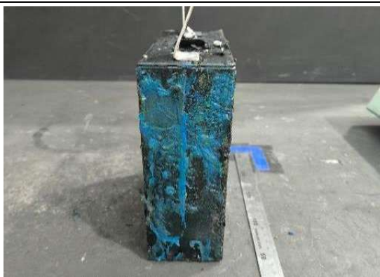
Figure 37: After thermal runaway-2
