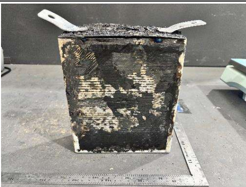
Figure 13: After thermal runaway-2
