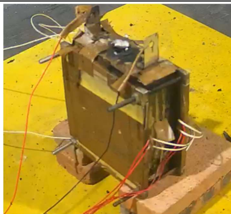
Figure 18: After thermal runaway-1
