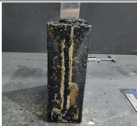
Figure 20: After thermal runaway-3
