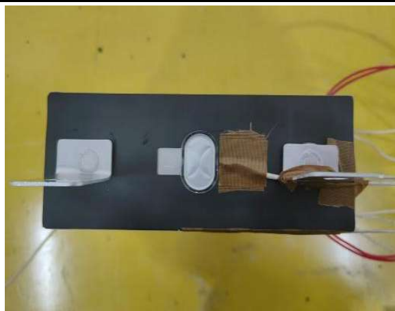
Figure 7: TC location near cell vent and positive node
