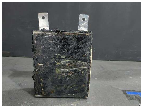
Figure 25: After thermal runaway-2
