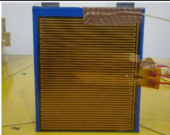
Figure 6: TC location on cell wide surface not covered by heater
