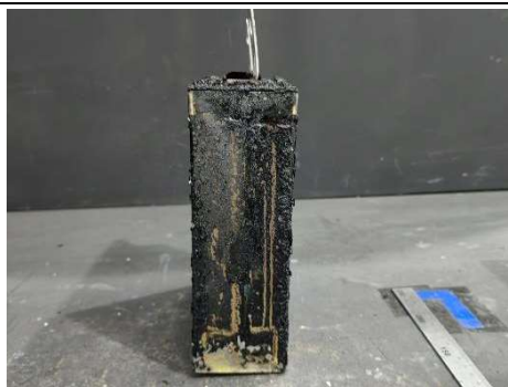
Figure 32: After thermal runaway-3
