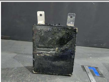
Figure 31: After thermal runaway-2
